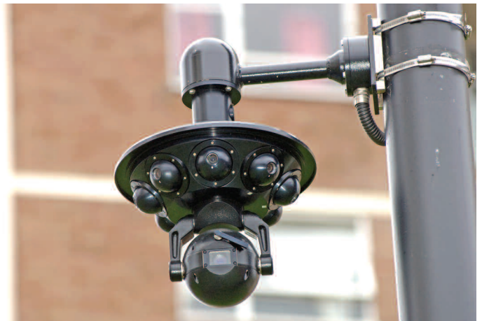
The Bug, a rugged version of Safetywatch, is virtually bomb-proof and has survived being blasted at point-blank range by a shotgun
